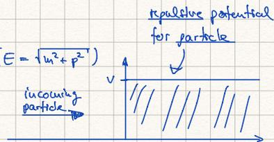
$$\left. \begin{array}{l} z < 0: [-E^2 - \frac{d^2}{dz^2} + m^2] \psi(z) = 0 \\ z > 0: [-(E-V)^2 - \frac{d^2}{dz^2} + m^2] \psi(z) = 0 \end{array} \right\} \begin{array}{l} \psi(z), \frac{d}{dz}\psi(z) \text{ continuous at } z=0 \\ (\text{because no } \delta(z), \delta'(z) \text{ in KG equations}) \end{array}$$
