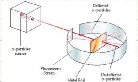
↳ classical mechanics:  $b = \frac{q_1 q_2}{8TE} \cot\left(\frac{\theta}{2}\right)$   $\leftarrow$  kinetic energy of incoming particle
