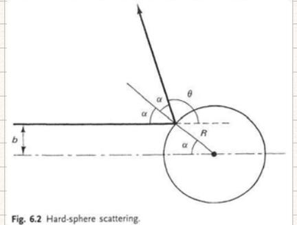
Fig. 6.2 Hard-sphere scattering.
