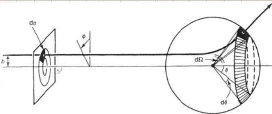
Fig. 6.3 Particle incident in area  $d\sigma$  scatters into solid angle  $d\Omega$ .
