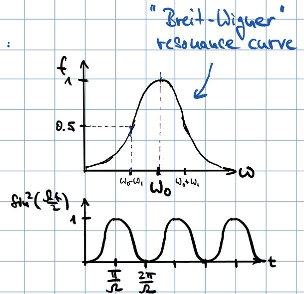
When the rotation frequency  $\omega$  is equal to  $\omega_0$  ("on resonance") the spin oscillates between the states "spin up in z-direction" ( $\begin{pmatrix} 1 \\ 0 \end{pmatrix}$ ) and "spin-down in z-direction" ( $\begin{pmatrix} 0 \\ 1 \end{pmatrix}$ ) with frequency  $\frac{2\pi}{\Omega}$ .
