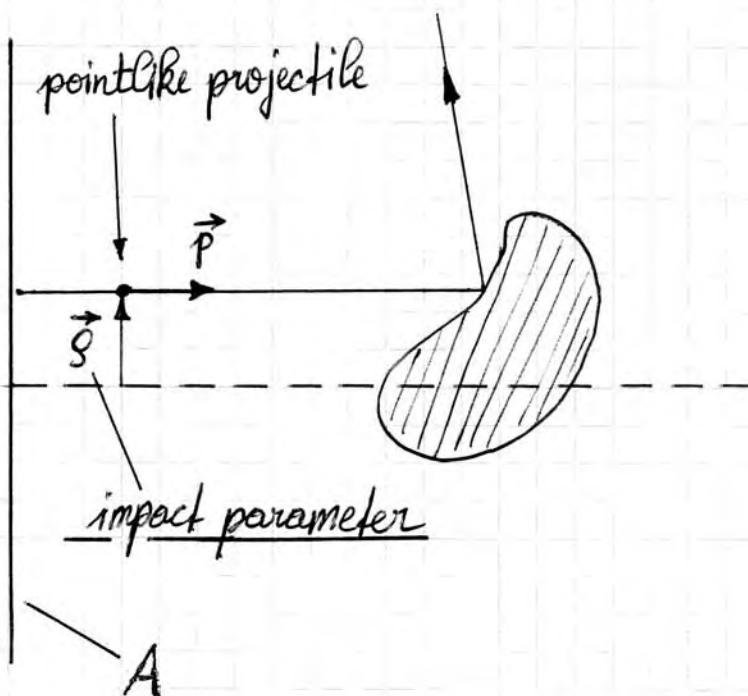
we repeat this experiment  $N$  times with randomly distributed impact parameter  $\vec{s}$  (area  $A$  larger than dimensions of the object)
