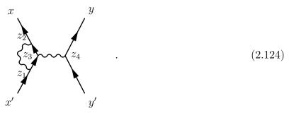
The extra photon propagator produces a vertex correction:
