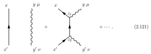
We may indeed use the same Feynman rules as for electron-electron scattering, because the electron that starts from x' and at  $z_2$  absorbs a photon, does not make a difference between a virtual photon (that will be absorbed further by an electron or positron or any other
